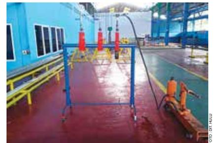
Alat pengetesan kebocoran *Standing Valve* di Pump Shop Rantau Field.
